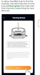
found it will show in your search results press on "Done" to complete the process. Dimmable light 1 15. If the dimming effect is not satisfactory press the button for 25 seconds to switch from trailing edge to leading edge. When the switch has been made, the LED indicator will flash once to indicate the dimmer is set to leading edge or twice for trailing edge.
